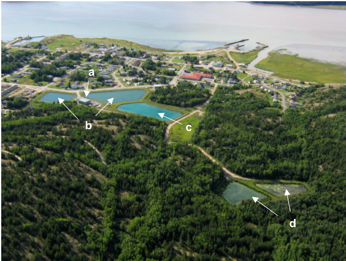
Figure 6. Location of the water treatment plant and ponds, 12 August 2006. a. The water treatment plant. b. Two reservoir ponds. c. Backwash pond. d. Two sewage ponds.
