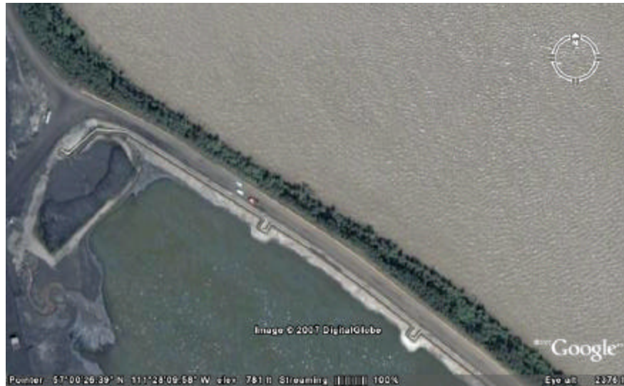
Figure 18. A visible-band satellite image of the Athabasca River and an adjacent Suncor tailings pond illustrates the dangerous juxtaposition of contaminated ponds (left) and the Athabasca River (right). Note the bright, wave-textured surface of the Athabasca River in comparison to the darker, smoother surface of the tailings pond. In a radar image, there could be a large contrast in the backscatter of the two water bodies. Image from Google Earth.
