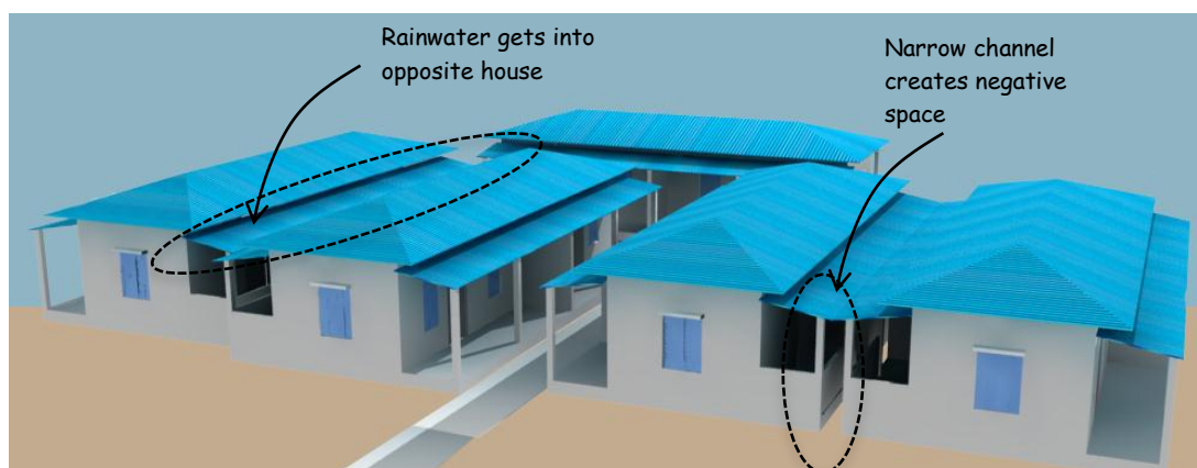
Figure 4.13: Faulty roofing system and wastage of space in a cluster in Mandartola settlement.
