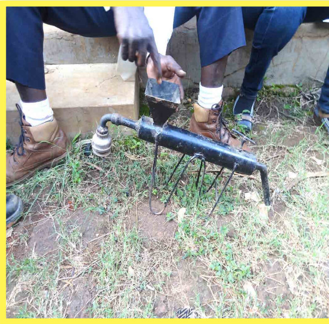
Plate 18: Types of retorts used in Busia District appropriate for burning and mercury amalgam
