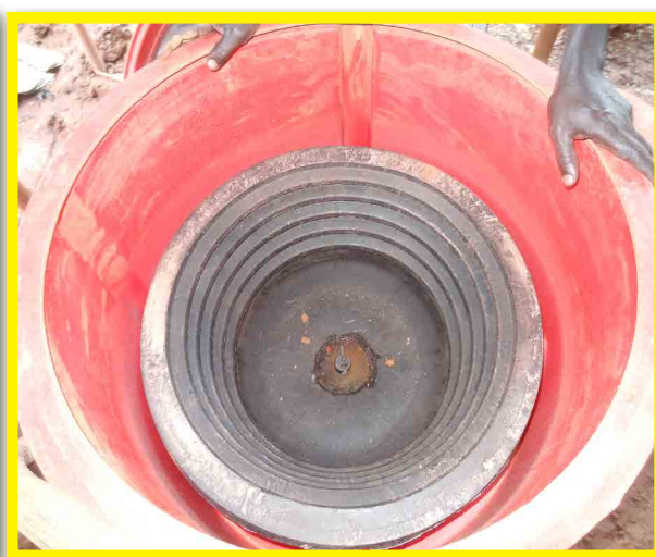
Plate 6: Use of centrifuge to concentrate gold in Busia District
